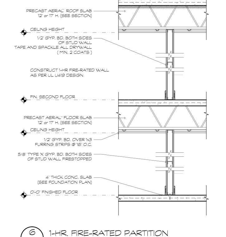
NOTE: INSTALL 3M FIRESTOP OR APPROVED EQUAL @ ALL WALL PENTRATIONS AS PER MANUFACTURERS SPECIFICATIONS
